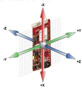
The module contains a 3D accelerometer (up to 16g), which can be used for a variety of custom specific (M2M) applications. Accelerometers are useful for measuring movement, speed, g-forces and vibration of the object. The accelerometer and advanced embedded firmware enables a very low-power battery solution.
